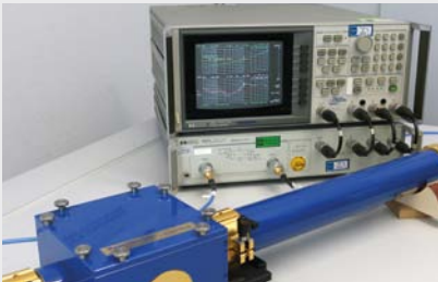
Coupling resistance, triaxial pipe
