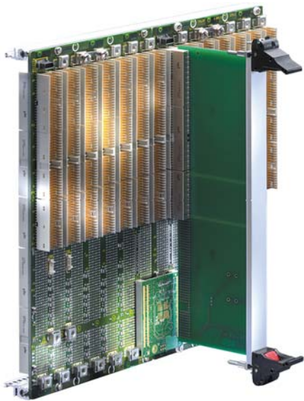
Photo shows primary and secondary backplane with inserted bridge and fitted rear transition board
