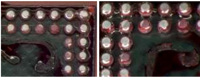
Figure 7: Cracks found at the top interconnect on both tack flux devices tested using dye and pry
