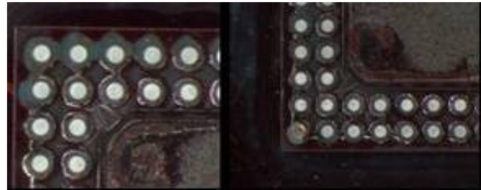
Figure 9: No cracks found on epoxy flux system
