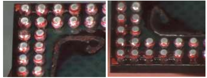
Figure 8: Cracks found on top interconnect only where there is an electrical failure at the top level for the solder dip process
