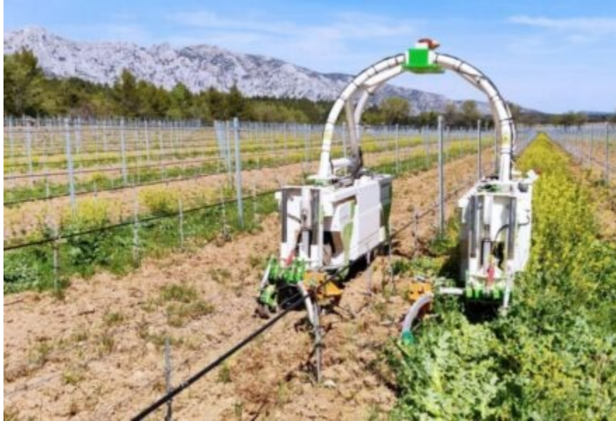
Figure 9: The naïo technologies “Ted” robot for agricultural applications with exchangeable tools such as finger hoes, disc lumpbreakers, serrated discs, and more. Source: naïo technologies
