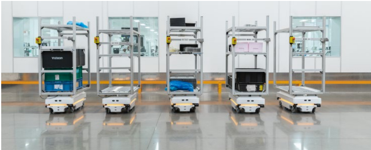
Figure 2: The MiR100 AMR from Mobile Industrial Robots (MiR) transporting raw materials from a warehouse to the production lines and returning with finished products. Source: MiR
