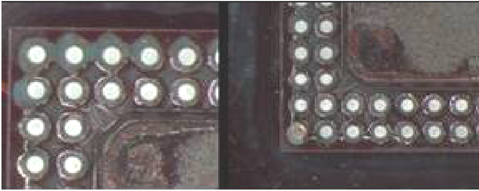
Figure 5. CSP device assembled using epoxy-flux technology (after reliability testing)
