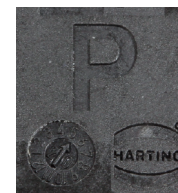
Date indicator in a P-module
