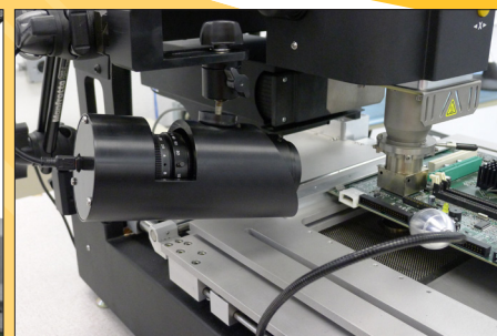
Side view camera for increased reflow visibility
